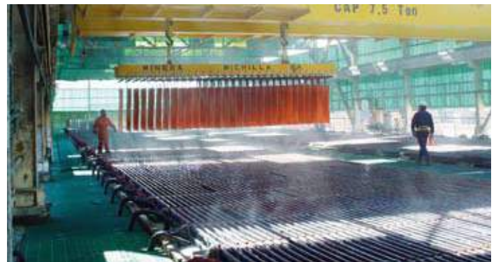
Copper cathodes in the electro-winning plant at Michilla
